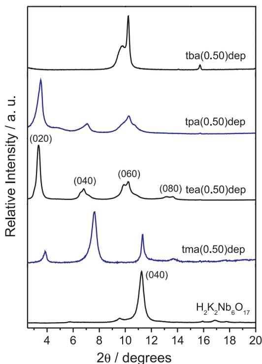
**Figure 3.** XRD patterns of  $\text{H}_2\text{K}_2\text{Nb}_6\text{O}_{17}$ , tma(0.50)dep, tea(0.50)dep, tpa(0.50)dep and tba(0.50)dep.
