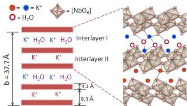
**Figure 1.** Representation of the  $K_4Nb_6O_{17} \cdot 3H_2O$  structure. In the right hand side, solid and dashed lines among the interlayer species and the  $NbO_6$  units represent the ionic interactions and hydrogen bonds.
